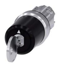
key-operated switch Siemens, 22 mm, round, metal, shiny, special lock, with 2 keys, 3 switch positions I-O-II, latching, actuating angle  $2x45^\circ$ , 10:30h/12h/13:30h, key removal II
