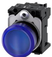
Indicator light, 22 mm, round, plastic, blue, lens, smooth, with holder, LED module with integrated LED 110 V AC, screw terminal, with laser labeling, upper case and lower case, always upper case at beginning of line
