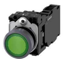
Illuminated pushbutton, 22 mm, round, plastic with metal front ring, green, pushbutton, flat, momentary contact type, with holder, 1 NO+1 NC, LED module with integrated LED 110 V AC, screw terminal, with laser labeling, upper case and lower case, Always upper case at the beginning of the word
