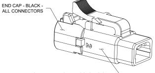
2 POS, PLUG, SOCKET, ATM SERIES, SNAP FIT
