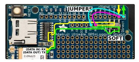
Yep - to use "hardware serial" the switch will be in the "soft serial" position.
