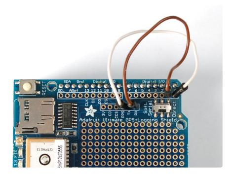
Finally upload the Adafruit\_GPS->leo\_echo sketch to the Leonardo, this will shuffle data from the GPS to the USB port
