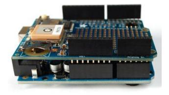
Fit the long pins through the pads until they slot into the Arduino. Depending on which version/type of Arduino you may need to use 2 x 8pin and 2 x 6pin or 1 x 10pin, 2 x 8pin and 1 x 6pin.
