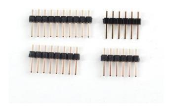
If you want to go with male headers, break off the 36-pin long stick into either 2 x 8pin and 2 x 6pin or 1 x 10pin, 2 x 8pin and 1 x 6pin (depending on how many headers your Arduino has and which version it is)
