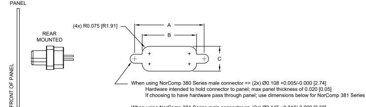
When using NorComp 381 Series male connector => (2x) Ø0.145 +0.010/-0.000 [3.68] Hardware intended to pass through panel
