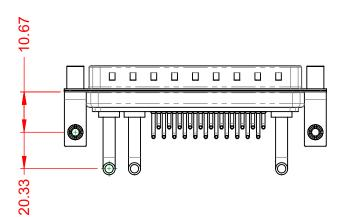
POWER/CO-AX CONTACT RATING:30A (CURRENT)(IF PRESENT)SIGNAL CONTACT CURRENT RATING:5A PER CONTACTSIGNAL CONTACT RESISTANCE:10mΩ MAX.INSULATOR RESISTANCE:5000MΩ min.DIELECTRIC5000MΩ min.
