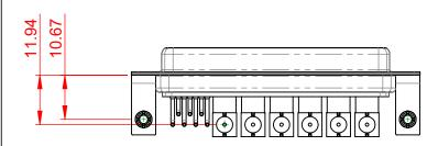
POWER/CO-AX CONTACT RATING: 75Ω (IMPEDANCE) (IF PRESENT) SIGNAL CONTACT CURRENT RATING: 5A PER CONTACT
