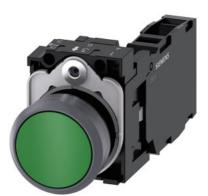
Pushbutton, 22 mm, round, plastic with metal front ring, green, pushbutton, flat, momentary contact type, with holder, 1 NO+1 NC, screw terminal, Z=20-unit packaging
