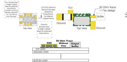
Attention: To achieve optimal frequency stability, and in some cases to meet the specification stated on this data sheet, it is required that the circuit connected to this TCXO output must have the equivalent input capacitance that is specified by the nominal load capacitance. Deviations from the nominal load capacitance will have a graduated effect on the stability of approximately 20 ppb per pF load difference.
