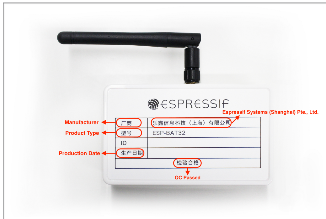
Figure 1-7. A Typical ESP-BAT32 Signal Board
