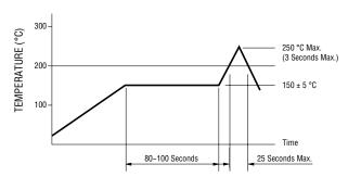
Processing Method: Reflow soldering with infrared heat (only once).
