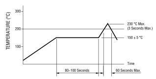
Processing Method: Reflow soldering with hot air (only once).
