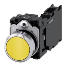
Pushbutton, 22 mm, round, metal, shiny, yellow, pushbutton, flat, momentary contact type, 1 NO+1 NC, Spring-type terminal
