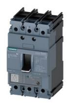
circuit breaker 3VA5 UL frame 125 3-pole, starter protection TM120M, AM, In=50A without overload protection short-circuit protection li=3...7 x In nut keeper kit on both sides
