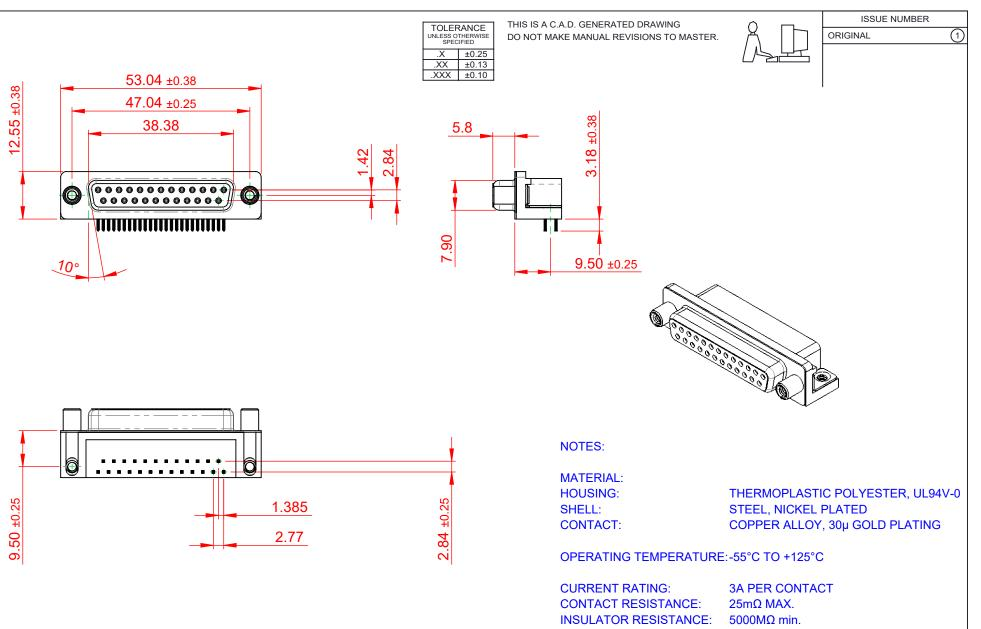
WITHSTANDING VOLTAGE: 1000V AC rms
