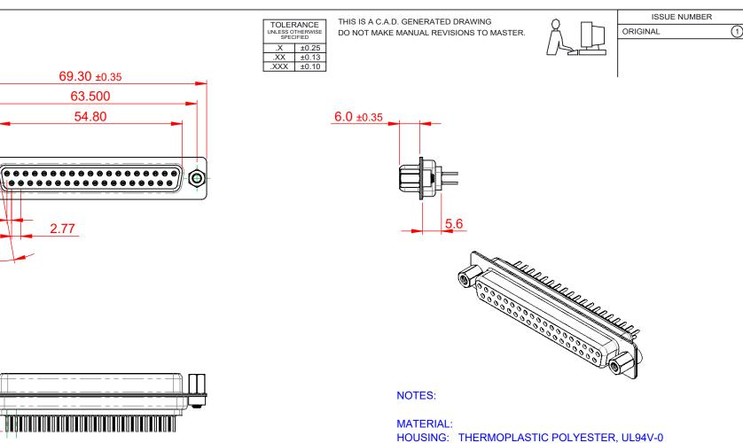
HOUSING: THERMOPLASTIC POLYESTER, UL94V-0 SHELL: STEEL, TIN PLATED CONTACT: COPPER ALLOY, 15µ GOLD PLATED OPERATING TEMPERATURE: -55°C to +105°C
