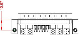
POWER/CO-AX CONTACT RATING: (IF PRESENT) SIGNAL CONTACT CURRENT RATING: 5A PER CONTACT SIGNAL CONTACT RESISTANCE:  $10m\Omega$  MAX.
