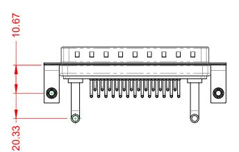
**OPERATING TEMPERATURE:** -55°C ~ 125°C 30A (CURRENT) **POWER/CO-AX CONTACT RATING:** (IF PRESENT) SIGNAL CONTACT CURRENT RATING: 5A PER CONTACT SIGNAL CONTACT RESISTANCE:  $10m\Omega$  MAX. **INSULATOR RESISTANCE:** 5000MΩ min. DIELECTRIC
