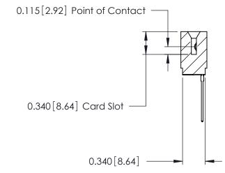
746 Series Ultra-Mate Card Edge Connector - Press Fit Part Number: 746-028-553-501 **EDAC INC** THESE DRAWINGS AND SPECIFICATIONS ARE THE PROPERTY OF EDAC INC.,AND TORONTO, ONTARIO SHALL NOT BE REPRODUCED, OR COPIED CANADA OR USED AS THE BASIS FOR THE MANUFACTURE OR SALE OF APPARATUS YOUR CONNECTION TO QUALITY & SERVICE
