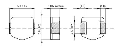
General Information Series MPX Style SMD Chip Size 0530(2120) Description Surface Mount Inductor Features Power Inductors **RoHS** Yes Core Composite Miscellaneous 40 (K) Temperature Rise Max.
