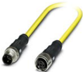
Sensor/actuator cable, 3-position, PVC, yellow, Plug straight M12 SPEEDCON, A-coded, on Socket straight M12 SPEEDCON, A-coded, cable length: 3 m
