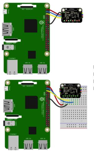
Pi 3V to sensor VCC (red wire) Pi GND to sensor GND (black wire) Pi SCL to sensor SCL (yellow wire) Pi SDA to sensor SDA (blue wire)
