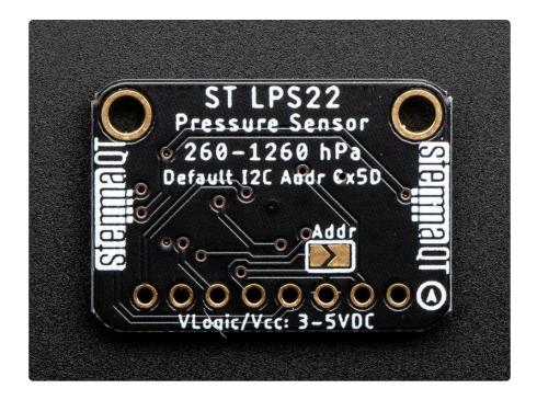
Furthermore, we've included <u>SparkFun Qwiic</u> () compatible <u>STEMMA QT</u> () connectors for the I2C bus so you don't even need to solder! All you need to do is plug in a <u>comp</u> <u>atible cable</u> (), wire it up to your device using one of our wiring diagrams and you're ready to write some code to start reporting measurements.
