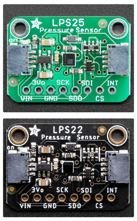
The LPS25 and LPS22 breakouts have identical pinouts; both boards are shown for reference
