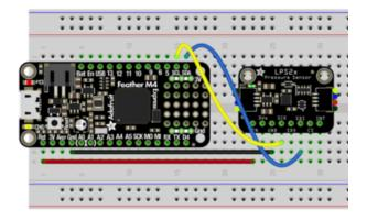
Board 3V to sensor VIN (red wire) Board GND to sensor GND (black wire) Board SCL to sensor SCL (yellow wire) Board SDA to sensor SDA (blue wire)
