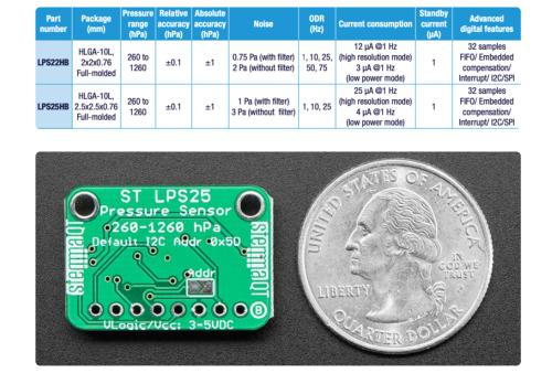
This table from an overview of ST's sensors shows how the two compare:
