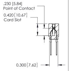
ACAD REFERENCE NO. 725-ENG MASTER 725 Series Ultra-Mate Card Edge Connector - Press Fit SEGAHOM:3A:9A DRAWN: J.LEE Part Number: 725-052-540-201 CHECKED: DATE: SCALE: **EDAC INC** SHEET 1 OF 1 THESE DRAWINGS AND SPECIFICATIONS ARE THE PROPERTY OF EDAC INC.,AND TORONTO, ONTARIO SHALL NOT BE REPRODUCED, OR COPIED DRAWING NUMBER **ISSUE** CANADA OR USED AS THE BASIS FOR THE 725-ENG MASTER MANUFACTURE OR SALE OF APPARATUS YOUR CONNECTION TO QUALITY & SERVICE WITHOUT WRITTEN PERMISSION.
