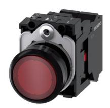
Illuminated pushbutton, 22 mm, round, plastic, red, pushbutton, flat, momentary contact type, with holder, 1NC, LED module with integrated LED 230 V AC, spring-type terminal, with laser labeling, upper case and lower case, always upper case at beginning of line
