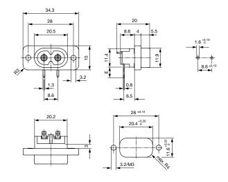
E = PCB terminal standard (additional solder): 6.9 mm
