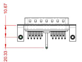
10A (CURRENT) **POWER/CO-AX CONTACT RATING:** (IF PRESENT) SIGNAL CONTACT CURRENT RATING: 5A PER CONTACT SIGNAL CONTACT RESISTANCE:  $10m\Omega$  MAX.
