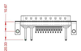
OPERATING TEMPERATURE: $-55^{\circ}C \sim 125^{\circ}C$ POWER/CO-AX CONTACT RATING:10A (CURRENT)(IF PRESENT)SIGNAL CONTACT CURRENT RATING:5A PER CONTACTSIGNAL CONTACT RESISTANCE:10m $\Omega$  MAX.INSULATOR RESISTANCE:5000M $\Omega$  min.DIELECTRICDIELECTRIC
