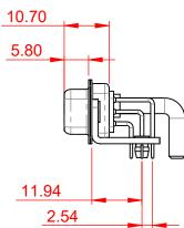
THERMOPLASTIC POLYESTER, UL94V-0 STEEL, NICKEL PLATED COPPER ALLOY, GOLD FLASH PLATED
