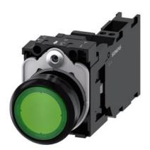
Illuminated pushbutton, 22 mm, round, plastic, green, pushbutton, flat, momentary contact type, with holder, 1 NO+1 NC, LED module with integrated LED 24 V AC/DC, spring-type terminal, with laser labeling, upper case and lower case, Always upper case at the beginning of the word
