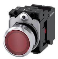
Illuminated pushbutton, 22 mm, round, Metal, shiny, red, pushbutton, flat, momentary contact type, with holder, 1 NC, LED module with integrated LED 230 V AC, spring-type terminal, with laser labeling, upper case and lower case, always upper case at beginning of line
