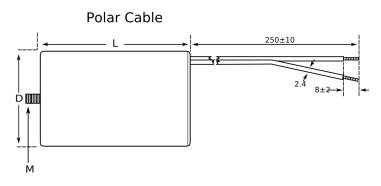
Series C28 Dielectric Film/Foil Polypropylene Style Plastic Case and Cover, Ultra Sonically Welded Description Ultra Sonically Welded Seal, Safety Class S3, UL\_94 V0 Disk **Features** RoHS Yes Termination Tin Copper Lead Cables UL, VDE, UL (Construction Only), UL\_94 VO Disk Qualifications AEC-Q200 Component 66.86 g Weight
