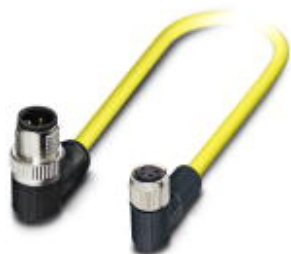
Sensor/actuator cable, 4-position, PVC, yellow, Plug angled M12 SPEEDCON, A-coded, on Socket angled M8, cable length: 1.5 m
