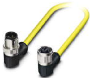
Sensor/actuator cable, 3-position, PVC, yellow, Plug angled M12 SPEEDCON, A-coded, on Socket angled M12 SPEEDCON, A-coded, cable length: 3 m
