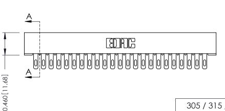
0.295 [7.49] Card Slot 0.090 [2.29] Point of Contact **SECTION A-A**
