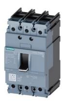
circuit breaker 3VA5 UL frame 125 breaking capacity class H 65kA @ 480 V 3-pole, line protection TM210, FTFM, In=100A overload protection Ir=100A fixed short-circuit protection li=10 x In UL489 SB (naval), 50 deg. cel. cable connection on both sides
