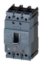
circuit breaker 3VA5 UL frame 125 breaking capacity class M 35kA @ 480 V 3-pole, line protection TM240, ATAM, In=15A overload protection Ir=12A ...15A short-circuit protection Ii=10...20 x In nut keeper kit on both sides
