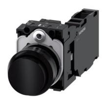
Pushbutton, 22 mm, round, plastic, black, pushbutton, raised, momentary contact type, with holder 1 NO+1 NC, screw terminal, with laser labeling, upper case and lower case, always upper case at beginning of line
