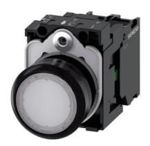
Illuminated pushbutton, 22 mm, round, plastic, white, pushbutton, flat, momentary contact type, with holder, 1NO, LED module with integrated LED 110 V AC, screw terminal, with laser labeling, upper case and lower case, always upper case at beginning of line
