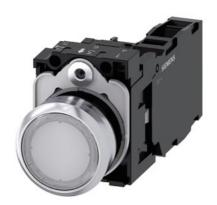
Illuminated pushbutton, 22 mm, round, metal, shiny, white, pushbutton, flat, momentary contact type, with holder, 1 NO+1 NC, LED module with integrated LED 24 V AC/DC, screw terminal, with laser labeling, upper case
