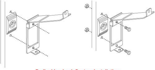
**Padlocking Lock System Installation**
