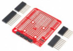
SparkFun Qwiic Shield for Arduino
