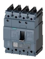
circuit breaker 3VA5 UL frame 125 breaking capacity class H 65kA @ 480V 4-pole, line protection TM230, FTAM, In=35A overload protection Ir=35A fixed short-circuit protection Ii=5...10 x In N conductor unprotected without connection
