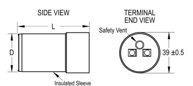
General Information Series MS/A902 Dielectric Aluminum Electrolytic Description Motor Start Aluminum Electrolytic RoHS Lead **Quick Connect** AEC-Q200 No Halogen Free Yes Component Weight 76 g Shelf Life 156 Weeks
