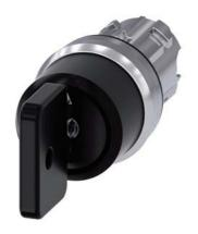
Key-operated switch O.M.R, 22 mm, round, metal, shiny, lock number 73034, black, with 2 keys, 3 switch positions I-O-II, latching, actuating angle 2x45°, 10:30h/12h/13:30h, key removal O, with laser labeling, inscription or symbol Customer-specific selection with SIRIUS ACT configurator (CIN)
