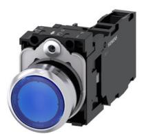
Illuminated pushbutton, 22 mm, round, Metal, shiny, blue, pushbutton, flat, momentary contact type, with holder, 1 NO+1 NC, LED module with integrated LED 230 V AC, screw terminal, with laser labeling, inscription or symbol Customer-specific selection with SIRIUS ACT configurator (CIN)
