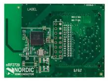
The module integrates all required external circuitry including a 16MHz crystal, matching network and a PCB quarter-wave antenna. The module also includes a 32kHz crystal that can be easily enabled or disabled with jumper settings. All chip I/O pins are made available on the module connector. The SMA module is identical except for the antenna being replaced with an SMA connector.
