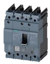
circuit breaker 3VA5 UL frame 125 breaking capacity class H 65kA @ 480V 4-pole, line protection TM230, FTAM, In=20A overload protection Ir=20A fixed short-circuit protection li=7.5...15 x In N conductor unprotected without connection
