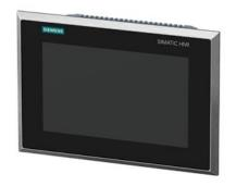
SIMATIC HMI TP900 Comfort INOX Stainless steel front, Glass pane, capacitive touch, Degree of protection front IP69K, 9" widescreen TFT display, PROFINET interface, MPI/PROFIBUS DP interface, 12 MB configuration memory, Windows CE 6.0, (Microsoft Support included Security updates discontinued) configurable from WinCC Comfort V15
