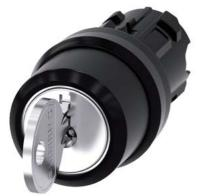
RONIS key-operated switch, 22 mm, round, plastic, special lock, with 2 keys, 3 switch positions I>O<II, momentary contact on the left, latching on the right, actuating angle 2x45°, 10:30h/12h/13:30h, key removal O, possible special locks: SB31, 421, 455
