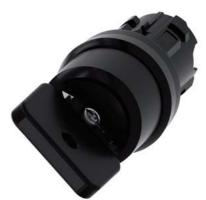
Key-operated switch O.M.R, 22 mm, round, plastic, lock number 73034, black, with 2 keys, 2 switch positions O<I, momentary contact type, Actuating angle 45°, 10:30h/12h, Key removal O Z=50-unit packaging
